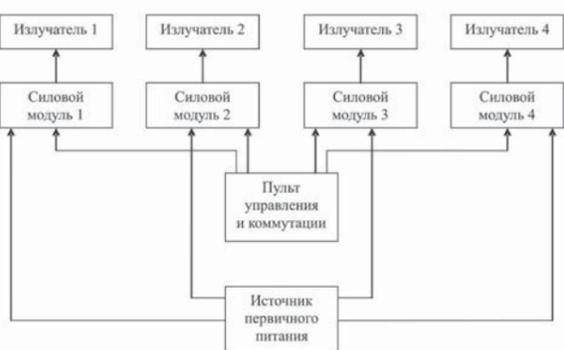
Schematic structural scheme of a super-power device. It is possible to create a super-power device for a total energy up to 200 kJ.
